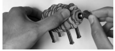
4. Using a penny or screwdriver, tighten the screw until it is snug. Be careful not to over tighten or you may move the gasket out of place.
